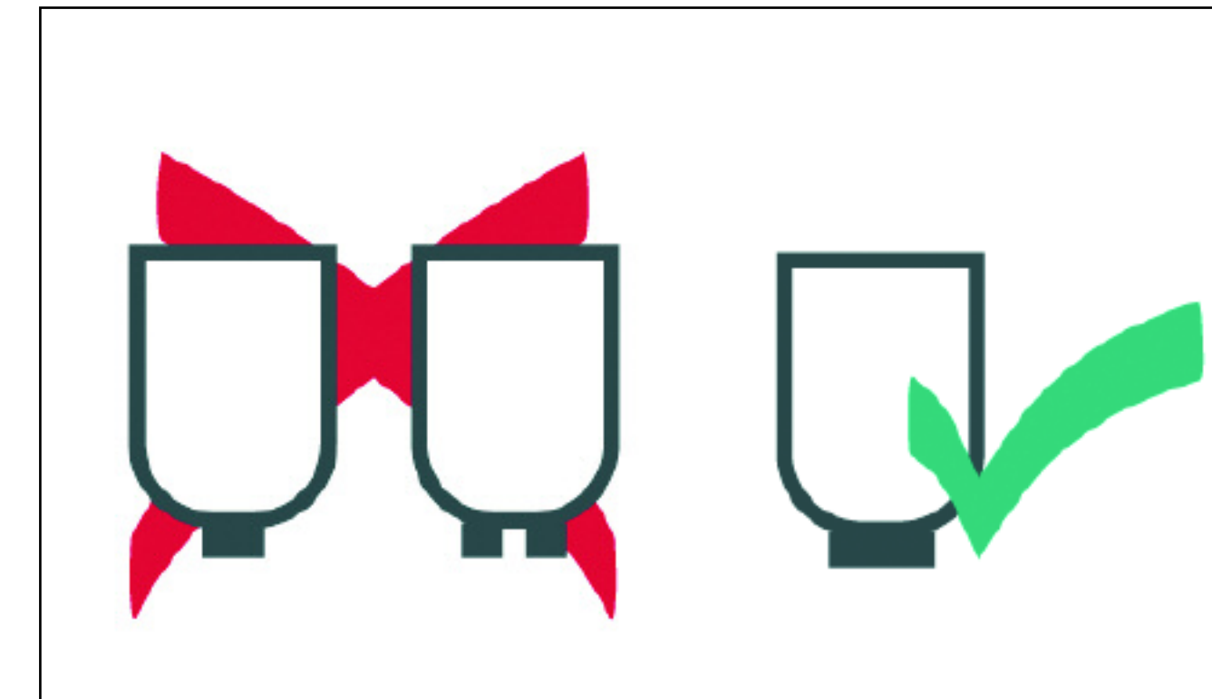
Base block must be flat, larger than crucible bottom and centered.
